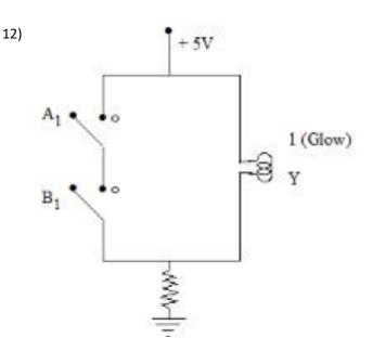
The logic gate equivalent to the given circuit diagram is :
